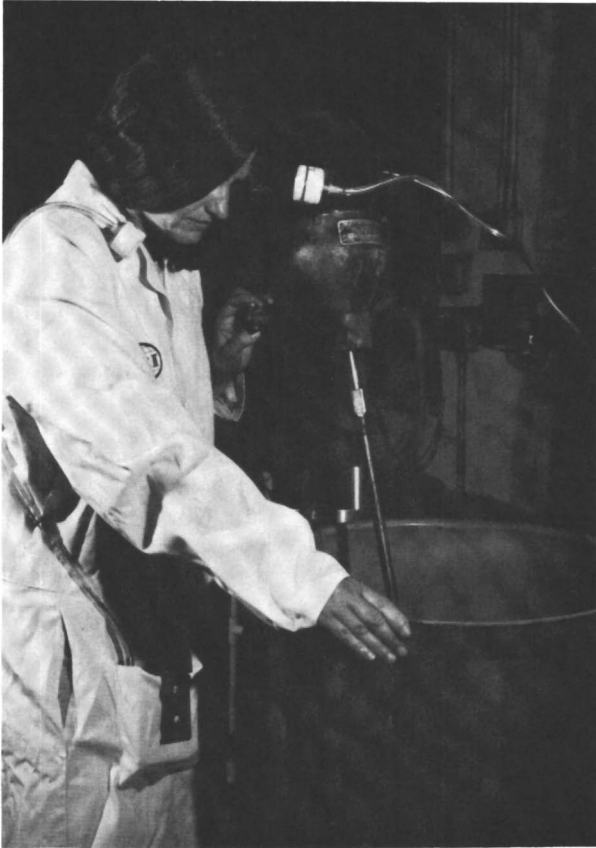
Figure 5. Here, a coat hanger has been modified to support an aerosol monitoring cassette and sampling hose.
