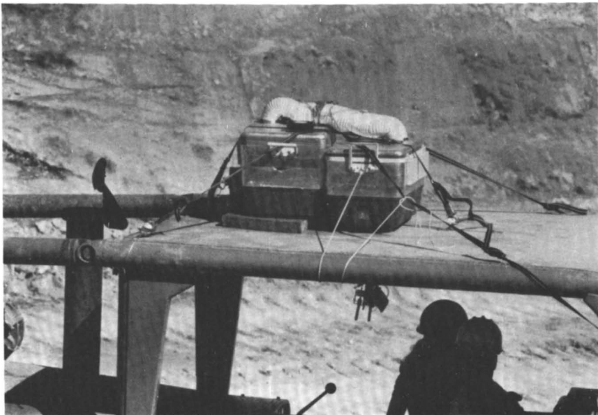
Figure 7. Securing instrumentation can pose problems under severe conditions. Here, webbing straps and rubber snubbers are used to secure instrument packages to earth-moving equipment.
