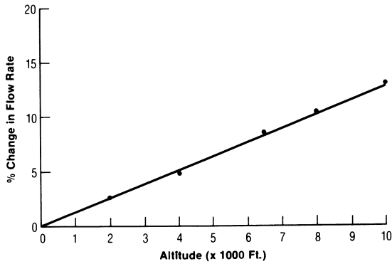
Figure 14. Altitude effect, pump model P-2500
